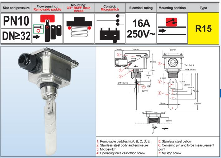
Main uses: Water flow detection on water pipes
